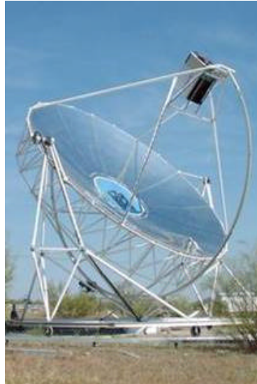
Parabolic Dish System
