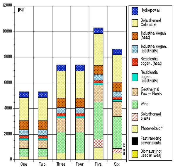
Pict. 2: Domestic gross energy production in petajoules using energy conversion technologies from renewable sources in Japan as used in the six scenarios. This is the production of electricity and heat in the installed power plants. Biomass, although listed is set to zero because of the unavailability of the potential of sustainable produced biomass.
