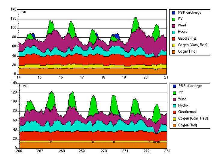
Pict. 4: The figures show the dynamics of electricity generation for 2 weeks of the year. The supply-system always produces enough electricity to cover the demand. If there is low electricity production of windenergy and photovoltaics at the same time, pumped storages get used to guarantee full supply (see days 14, 18, 19 and 271).
