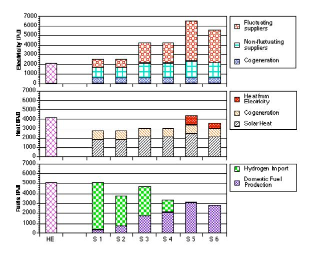
Pict. 3: Electricity, heat and fuel production in all six "Energy-Rich Japan" scenarios. Electricity surplus is used for heat and fuel production.Biomass, although listed is set to zero because of the unavailability of the potential of sustainable produced biomass.
